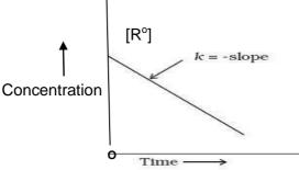
Example for zero order reaction is the decomposition of gaseous ammonia on a hot platinum surface at high pressure.
